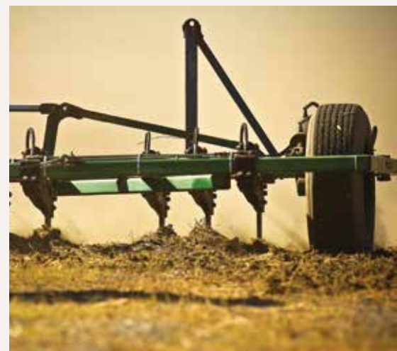
Deep rippers are commonly used to ameliorate compacted soils in particular to improve moisture penetration but, as yet, their effect on soil nutrients is not well known.
