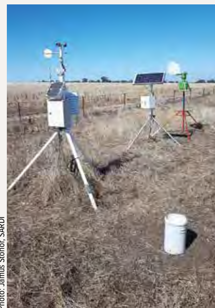
Spore trap and associated automatic weather station at Bordertown in 2018.
