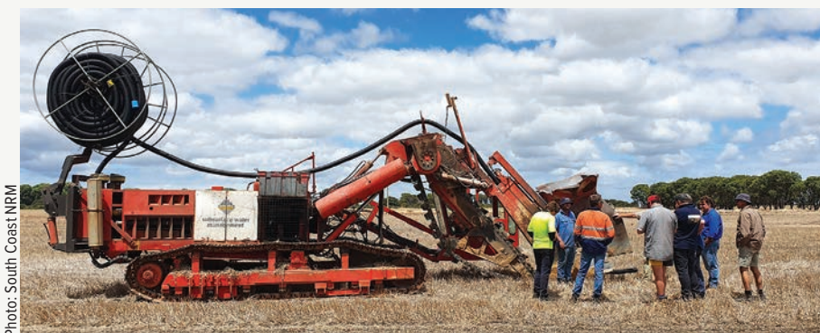
South Coast growers at the first installation of the tile drain in February 2020, with drainage contractor Subsurface Water Management.
