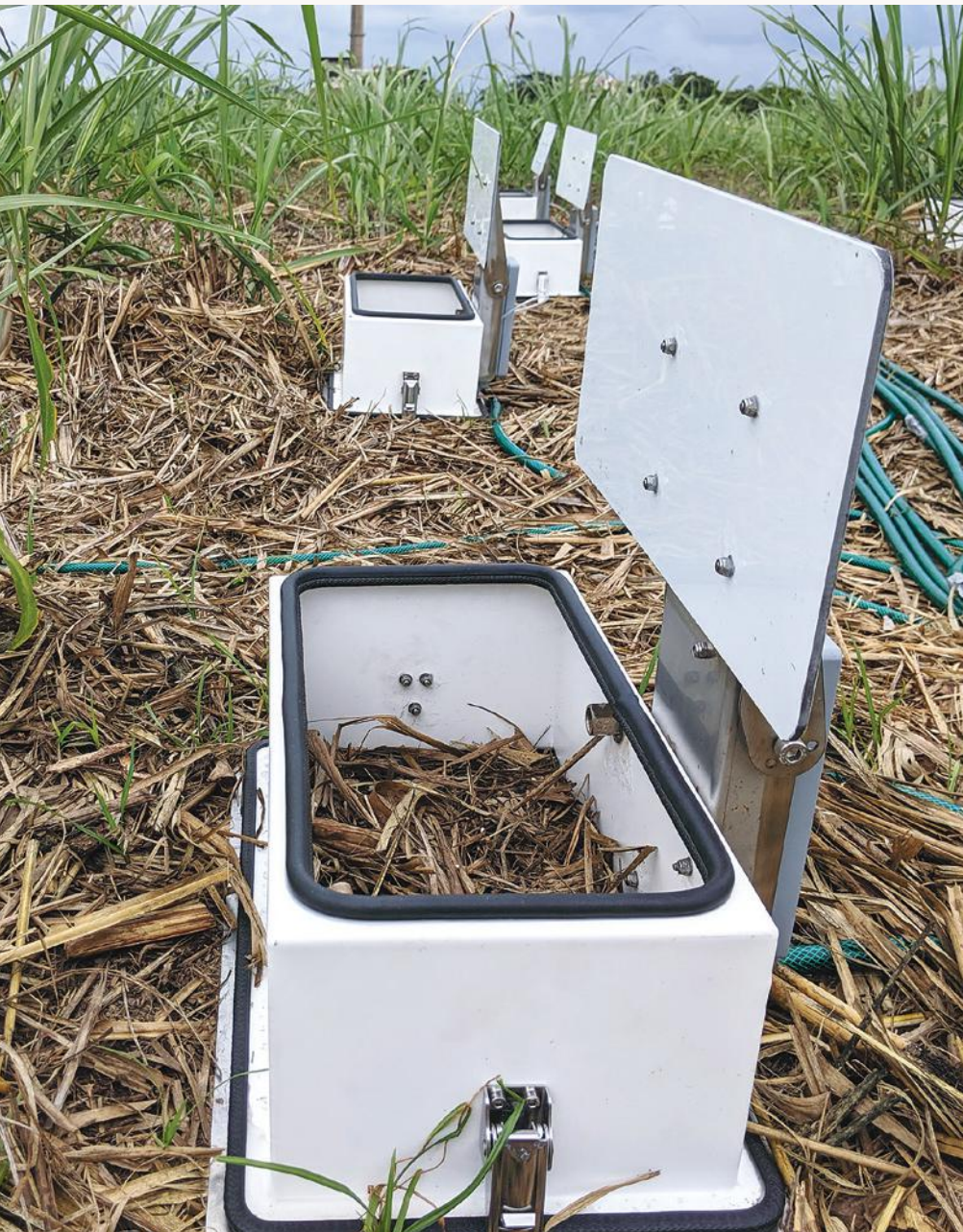
Field collection chambers are used to capture gaseous losses from denitrification. The lids are closed during the monitoring period.
