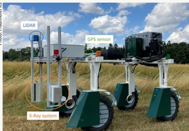
Figure 1: Phenotyping platform with different sensors: X-ray system, LiDAR and RTK-GPS sensor for use in canola.
